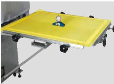
conventional mechanical fabric stretching systems, this unique fabric locking device reduces massive fabric waste, which is normally used just for clamping. To improve registration accuracy, 8 independent stretching knobs are provided to set optimum tension for wrap and weft thus enables to set even tension all over the screen.
