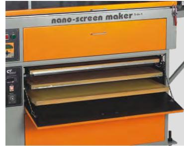
The thermal insulation is sandwiched between solid steel fabricated drying cabinet to retain heat inside the dryer.
